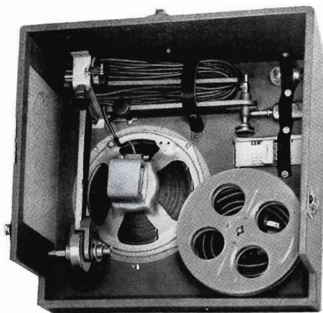
This sturdily built speaker case houses the 8" PM speaker and accessories
